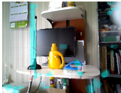
(b) The camera position is changed and the grasp affordance is not updated
